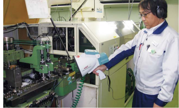
Air leak inspection
