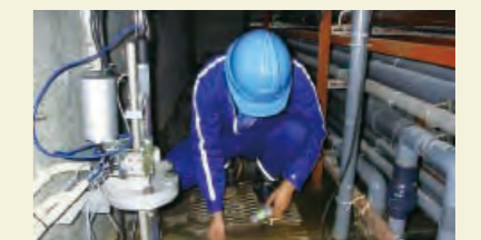
Using a measure to check the pH of waste water in a combined-use channel
