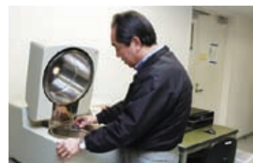
Verification testing using samples (fluorescent x-ray analysis)
