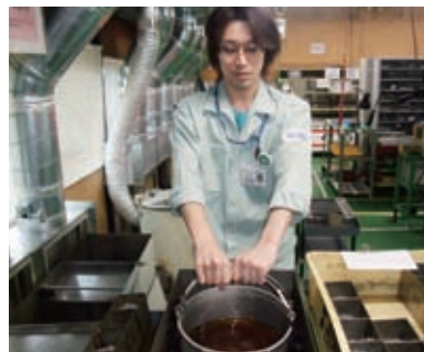
Washing watch components using functional water
