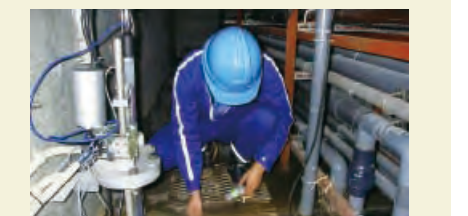
Using a measure to check the pH of waste water in a combined-use channel
