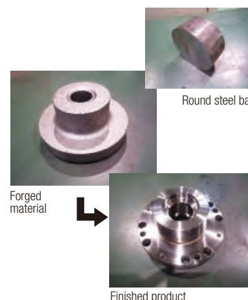
Reducing chips by forging materials
