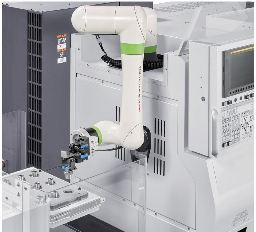
An on-machine-type robot system.
