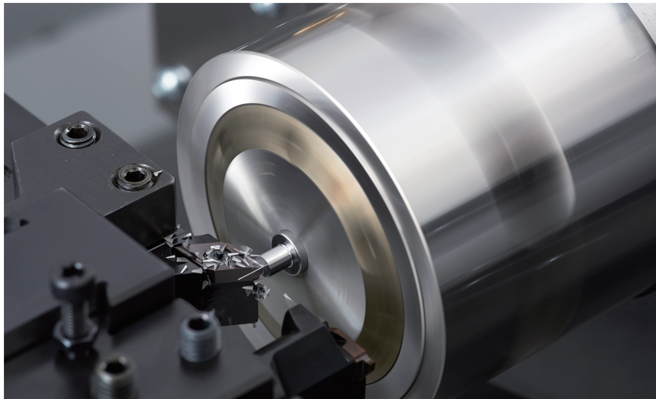
Microfabrication that leaves \phi 0.2 mm using low frequency vibration (LFV) cutting technology
