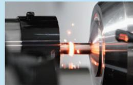
CITIZEN developed a technology called friction bonding that drastically reduces the amount of leftover materials after machine processing. This has reduced material costs and contributed to more environmentally friendly production.
