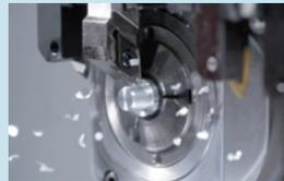
CITIZEN developed LFV (low frequency vibration) cutting technology, which reduces problems in production processes and contributes to improved productivity.
