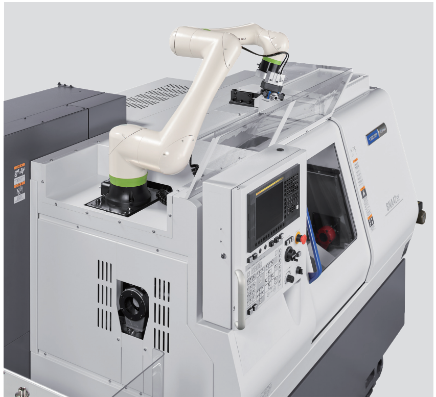
An on-machine-type robot system.
